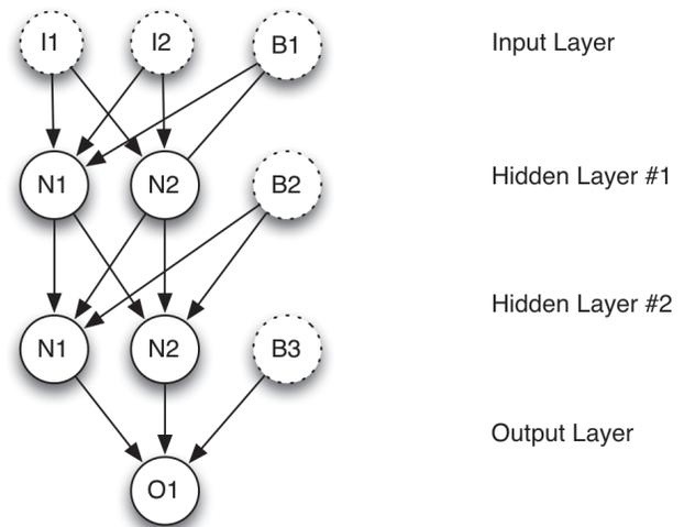
The above diagram shows how the biases (indicated by B's) are added to each of the layers.
