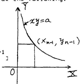
Instead of using a tangent, (9) suggests that we use the hyperbola  $xy = a$  to first obtain  $y_{n-1}$  from  $x_{n-1}$  and then make appropriate shifting and enlargement to arrive at  $x_n$ .
