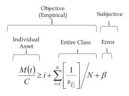
Where  $T_1$ ,  $T_2$ ,  $T_3$ ,... $T_N$ , are empirical ages at the time of replacement of assets from a class (asset mortality data), such as locomotives, gas turbines, or, even better, a homogeneous ensemble of similar vehicles in a fleet owned by the same enterprise. As soon as this inequality is satisfied for an individual asset, one must replace the asset in order to minimize costs for the entire class of assets.
