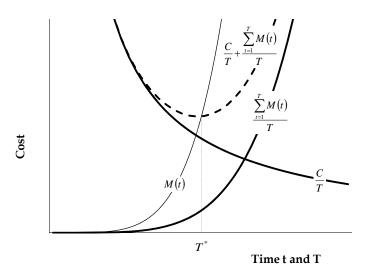
This graph shows the algebraic relationships of the first graph. The optimization problem is to maintain Average Total Cost at its minimum by correctly timing the replacements of individual assets.
