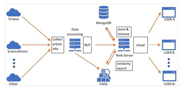
Generally, the system is composed of a data collection unit, an NLP unit, a document-oriented database, an indexing system, and a web server. Each of the components is described in the following sections.
