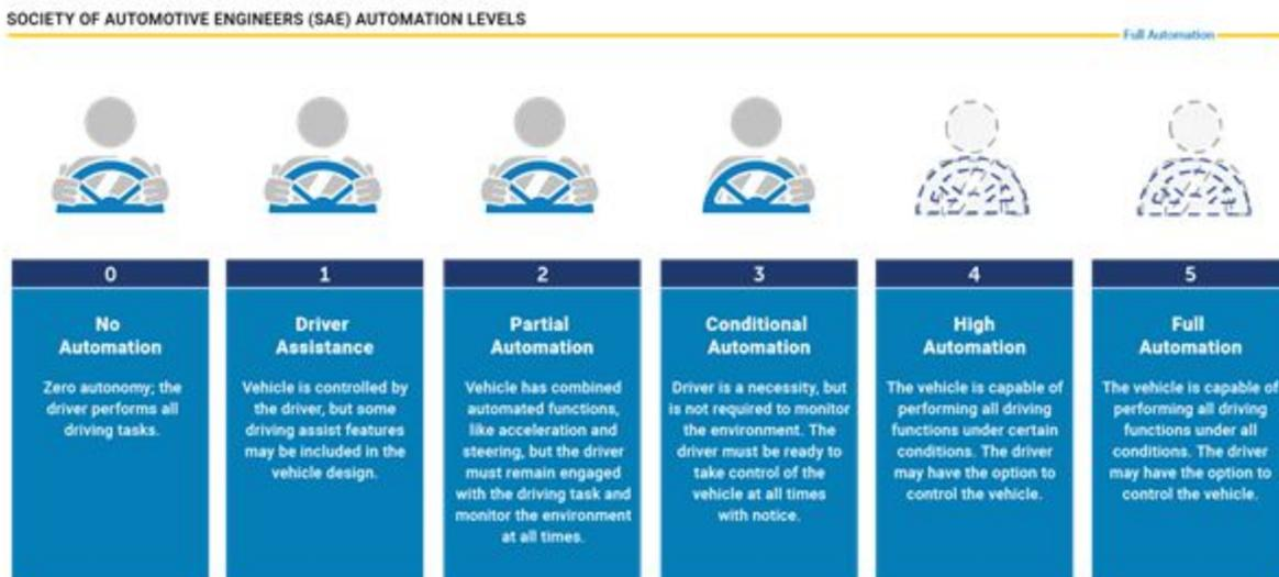
**Figure 2.2 Levels of Automation Source: NHTSA, 2018**
