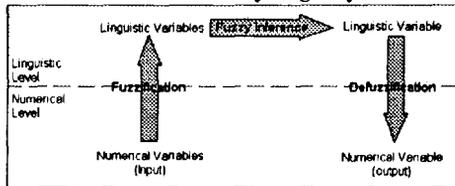
As indicated in the figure, the input of the system are numerical variables. These variables are passed through a fuzzification stage, where they are transformed to linguistic variables and subjected to inference rules. The logistics results are then transformed by a defuzzification stage into numerical values which become the output of the system.
