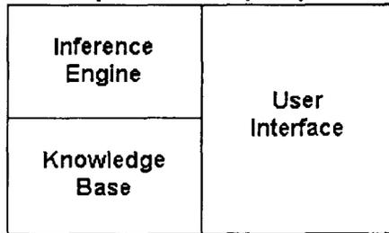
Briefly, the knowledge base contains the rules and facts about a certain domain, the inference engine uses the encoded knowledge to form inferences and draw conclusions, and the user interface provides facilities for such things as data input, reporting, graphical displays, explanations and on-line help systems.
